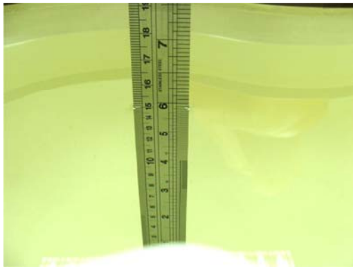
Fig 6.1 Photo of Liquid Height for Head SAR
