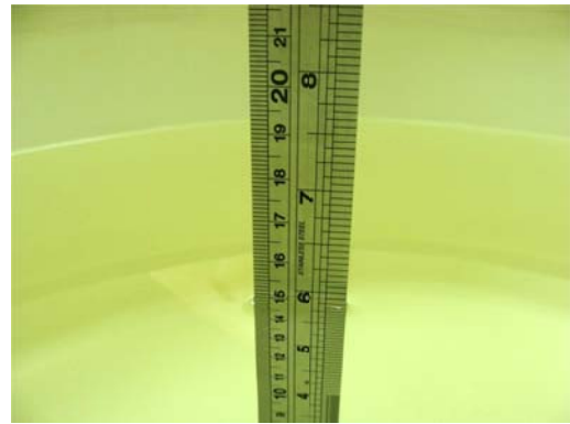
Fig 6.2 Photo of Liquid Height for Body SAR
