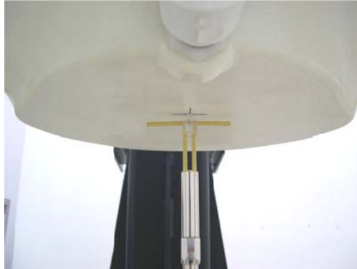
Fig 7.2 Photo of Dipole Setup
