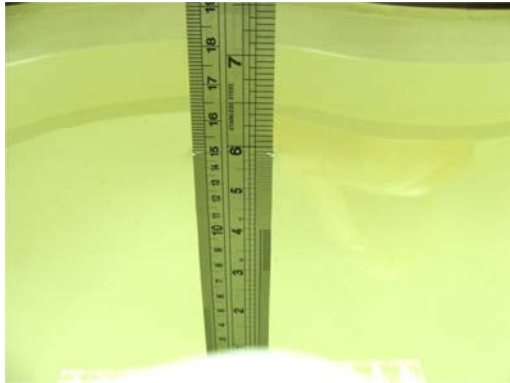
Fig 6.1 Photo of Liquid Height for Head SAR
