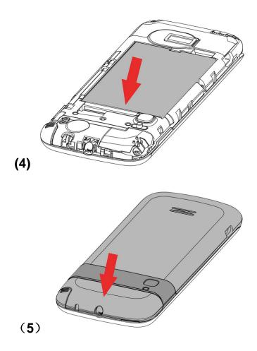
Note: make sure that the metallic contacts of the battery are facing the metallic contacts in the battery slot.
