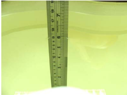
Fig 6.1 Photo of Liquid Height for Head SAR
