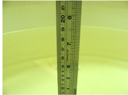
Fig 6.2 Photo of Liquid Height for Body SAR
