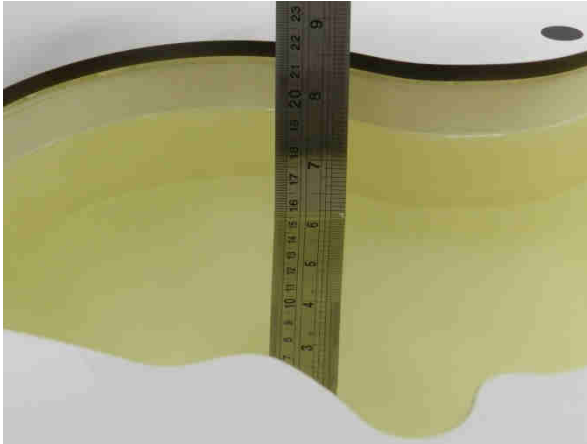
Fig 10.1 Photo of Liquid Height for Head SAR
