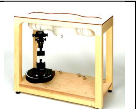
Fig 5.6 Photo of SAM Phantom
