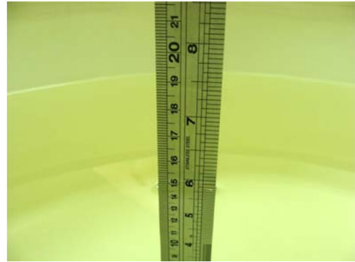
Fig 6.2 Photo of Liquid Height for Body SAR
