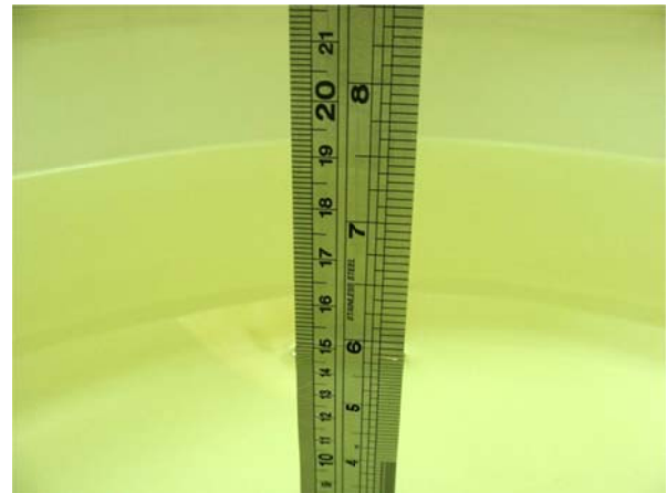
Fig 6.2 Photo of Liquid Height for Body SAR
