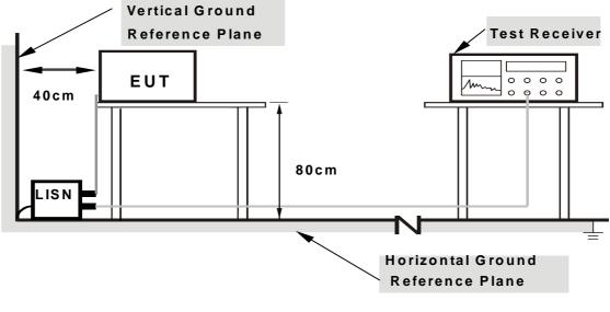
Note: 1.Support units were connected to second LISN. 2.Both of LISNs (AMN) are 80 cm from EUT and at least 80 from other units and other metal planes
