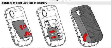
Removing the Battery and the SIM Card
