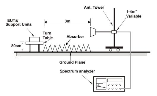
\*: depends on the EUT height and the antenna 3dB beamwidth both, refer to section 7.3 of CISPR 16-2-3.
