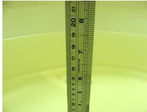
Fig 6.1 Photo of Liquid Height for Body SAR
