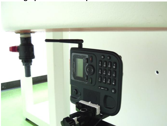
Vertical Antenna with 2.5 cm Gap
