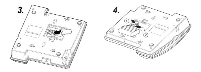
Note: The battery pack is a backup for emergencies in case of a power failure. Do not operate the phone without having the AC/DC adaptor connected. Be sure to carefully match the positive and negative terminals as shown on the battery.
