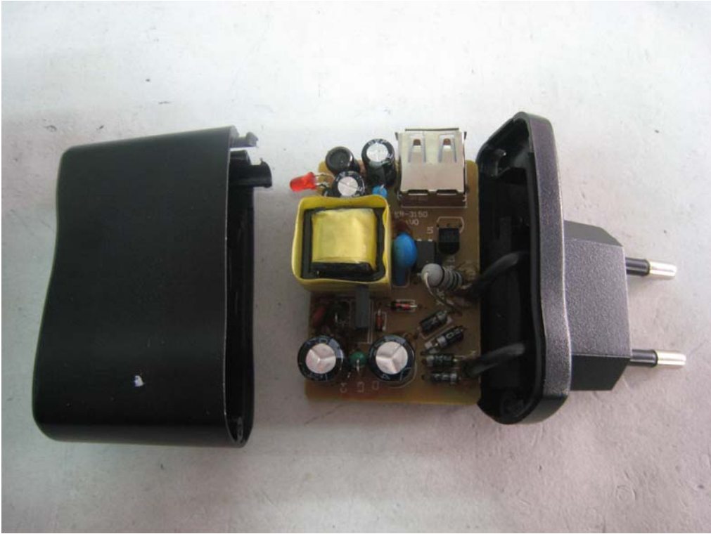
INTERNAL PHOTO OF POWER SUPPLY-1
