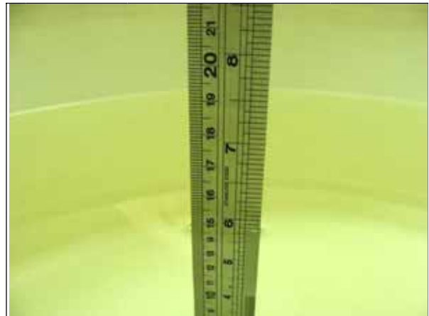
Fig 6.2 Photo of Liquid Height for Body SAR
