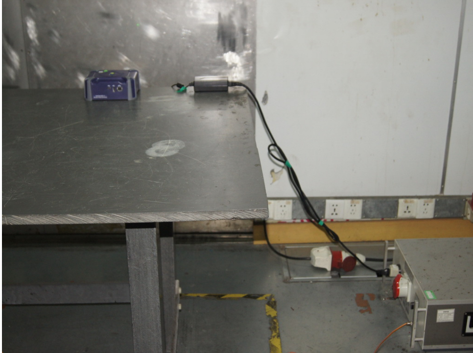
Photograph 7: Set-up for Conducted emissions
