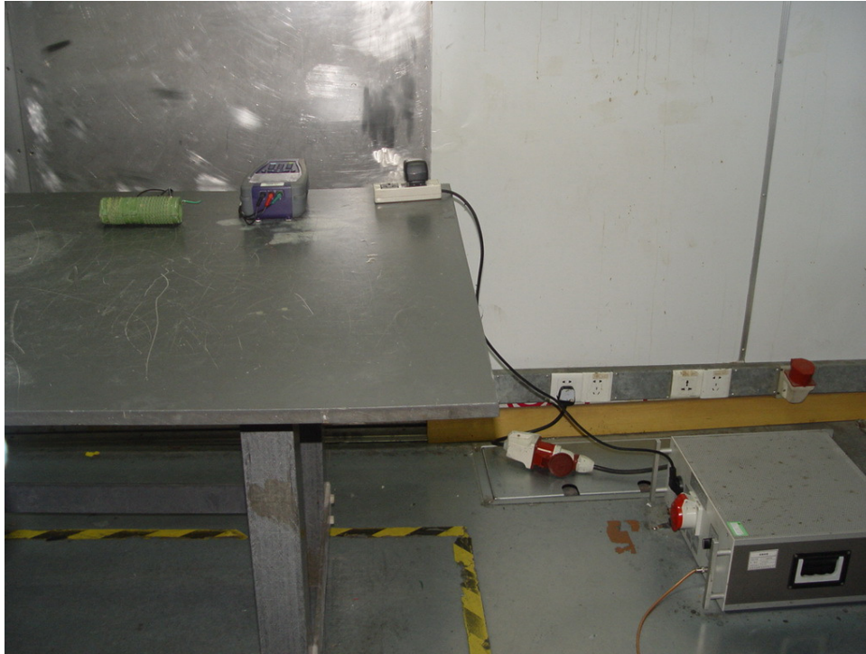
Photograph 5: Set-up for Conducted emissions
