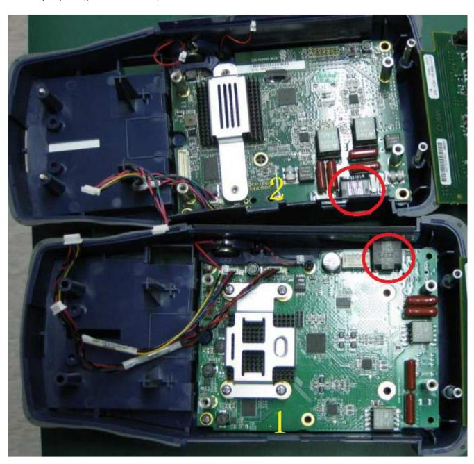
So 2 variants' overlay is a little different because of DSL port's position. Left overlays:
