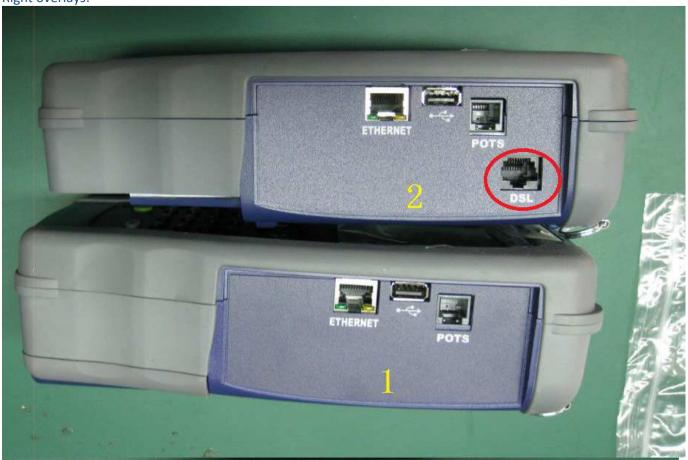
Variant 3 is thin revision to Variant 1, it only have top and bottom board inside, use a EMI shield to replace middle measurement board. So Variant 3 doesn't have top 3 jacks and right side's POTS port.
