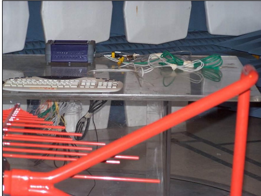
Photograph 2. Radiated Emission, Test Setup, 30 MHz to 1 GHz
