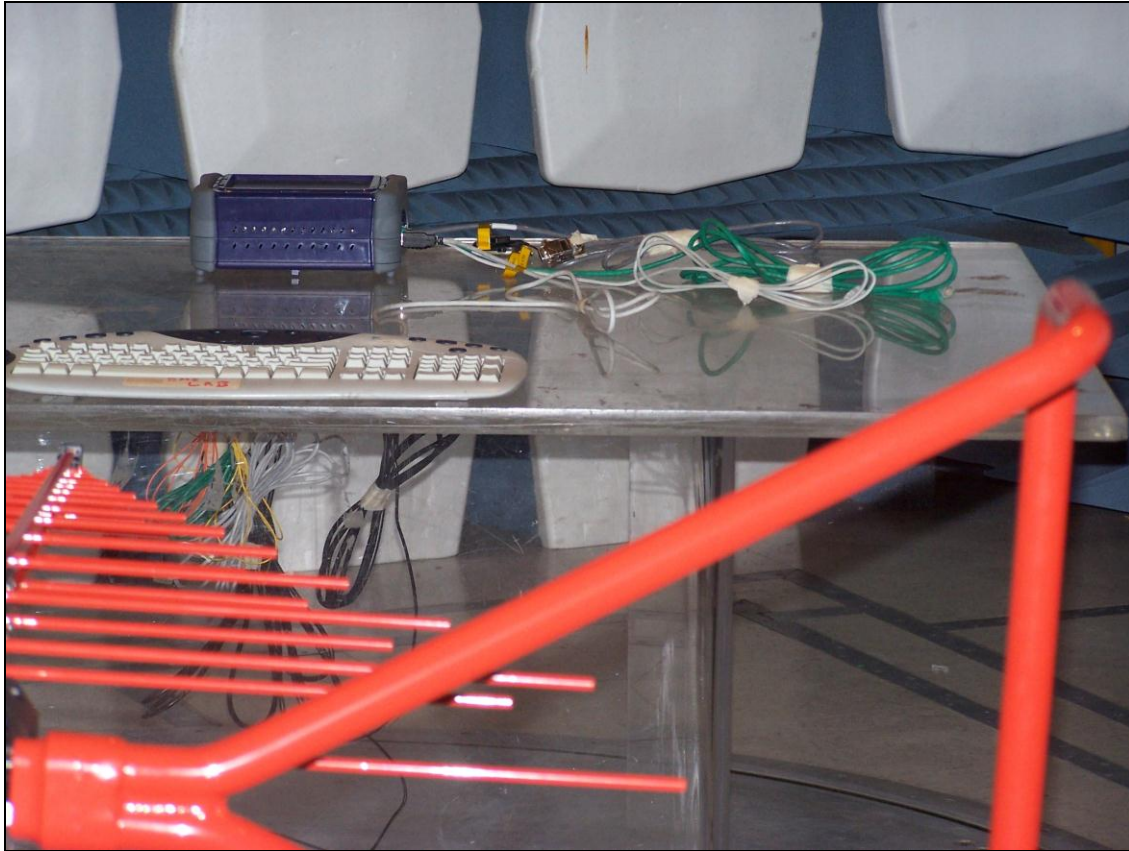
Photograph 2. Radiated Emission, Test Setup, 30 MHz to 1 GHz
