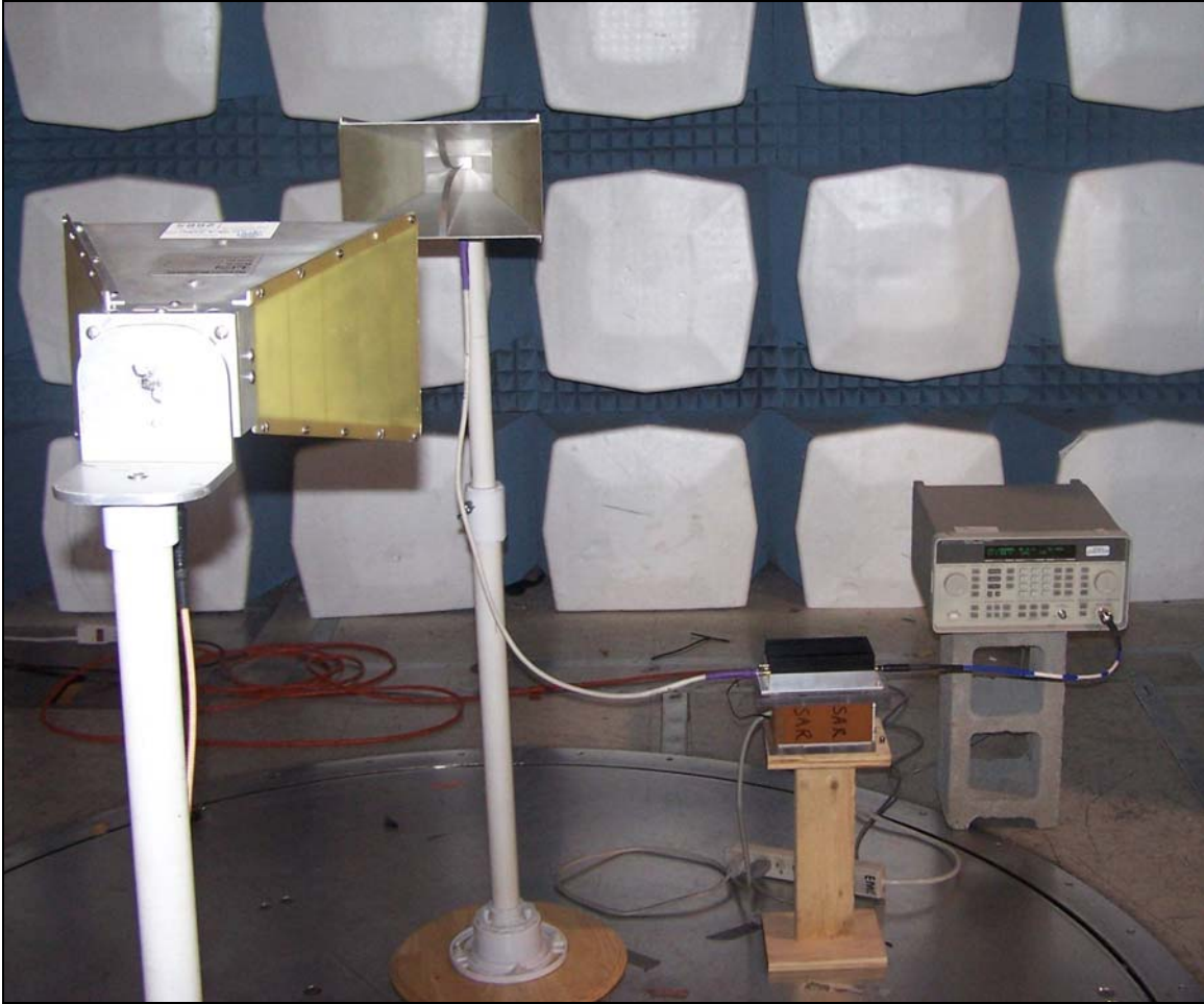
Photograph 3. 1900 MHz Antenna Substitution
