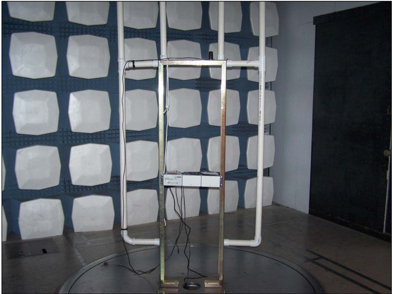
Photograph 2. Radiated Emission Limits Test Setup
