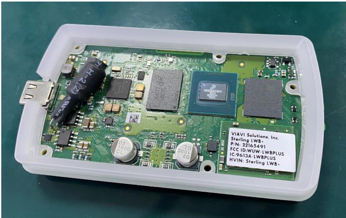
Picture#4, Put the light pipe on board it's has gap between label and edge of light pipe
