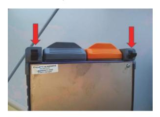
5 Insert the module hinges into the instrument at about a 45 to 60 degree angle.
