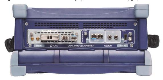
Figure 27 DMC with CSAM inserted (left) and MSAM v2 inserted (right)
