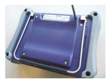
3 Lift off the back cover to expose the connector.
