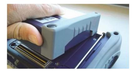
7 Seat the module into the connector with slight pressure.
