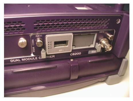
**6** Push the PIM into the port until the PIM panel is flush with the exterior panel of the chassis, and the PIM ejection button pops out.
