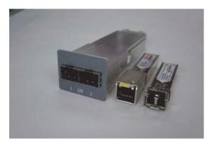
If you are inserting an XFP PIM, it requires a high rate MSAM chassis. These chassis are labeled with a C1000, C1004, C0400-v2, C0404-v2, or C1010-v2 model number on the exterior panel. After verifying that the chassis can support the PIM, look at the PIM label to verify that it is an XFP PIM.
