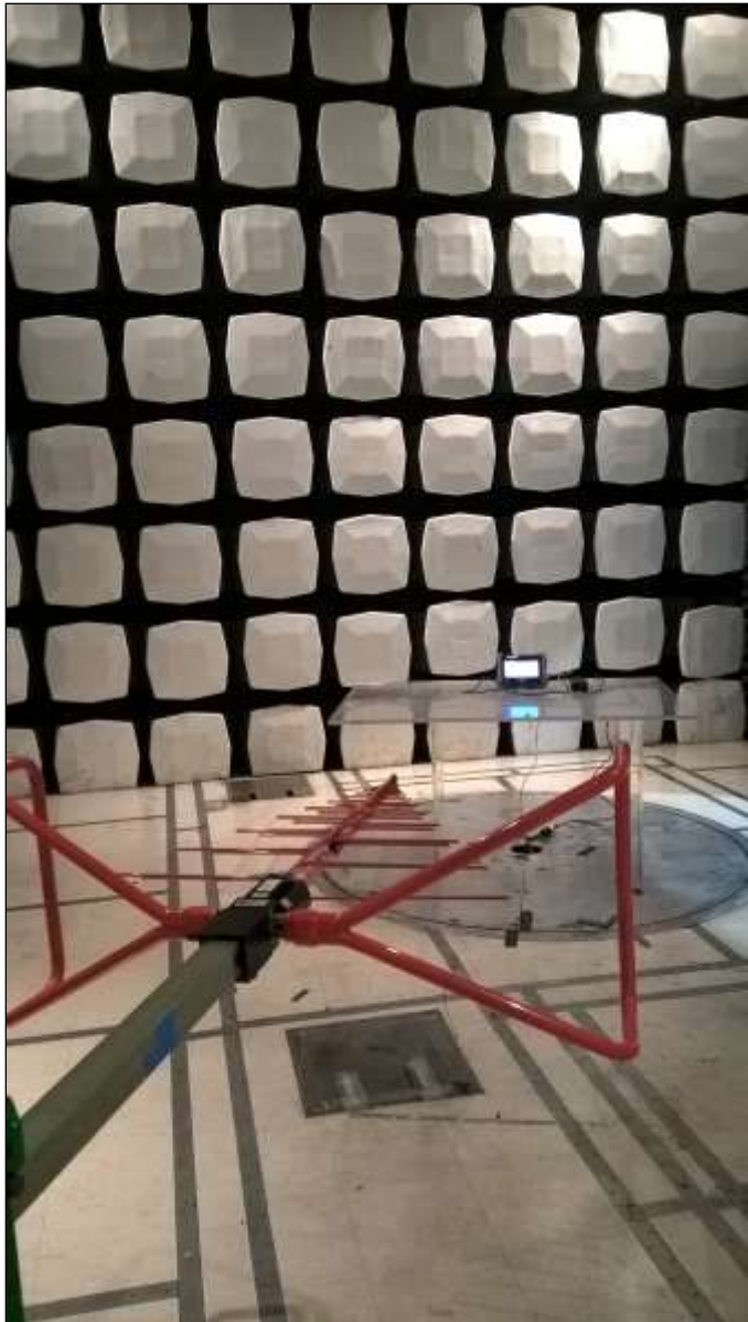
Photograph 2. Radiated Spurious Emissions, Below 1 GHz, Test Setup
