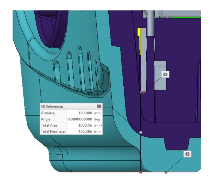
Antenna PCB Top To Front Contour
