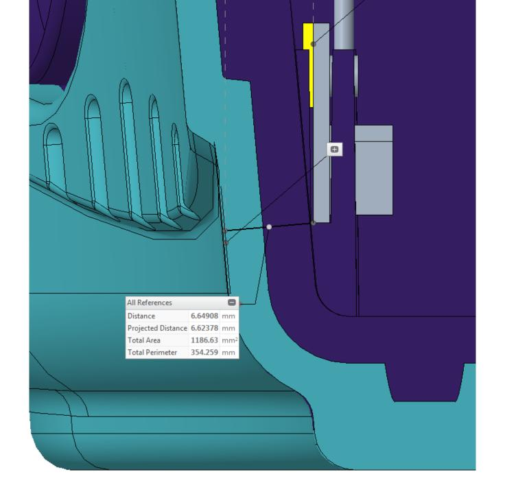
Antenna PCB Bottom To Rear Contour
