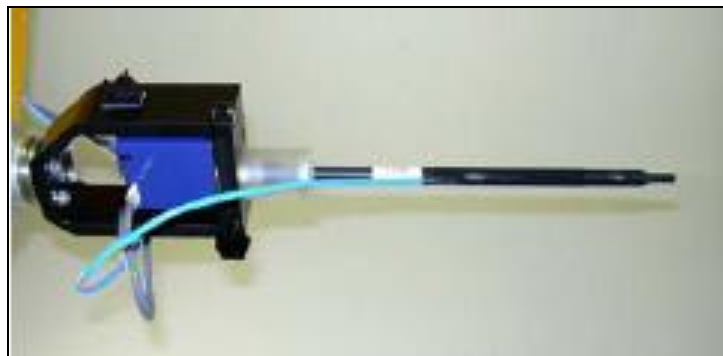
Figure 12: Electric field probe
