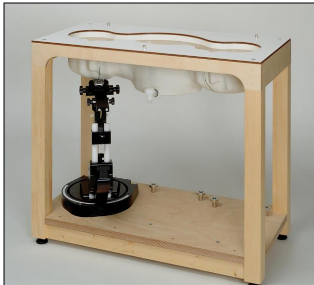
Figure 13: Specific anthropomorphic mannequin twin phantom
