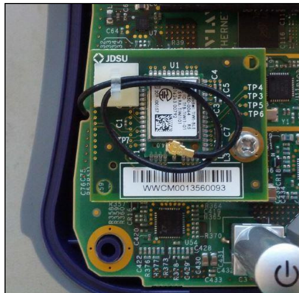
Figure 3: Antenna cable connection.
