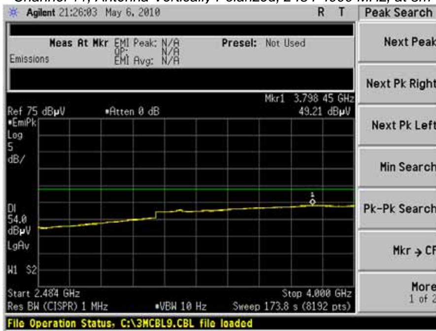
Channel 11, Antenna Vertically Polarized, 2484-4000 MHz, at 3m
