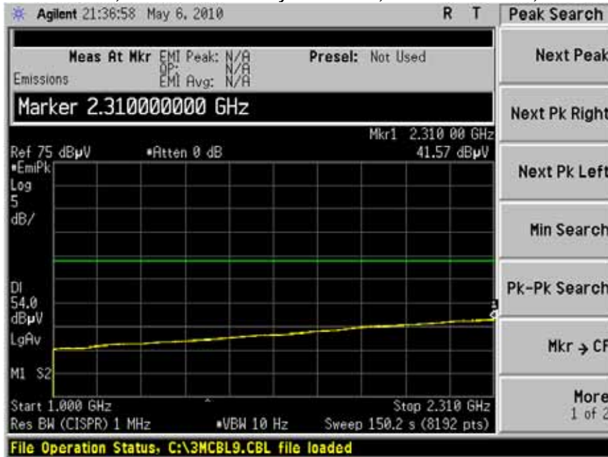
Channel 1, Antenna Vertically Polarized, 1000-2310 MHz, at 3m
