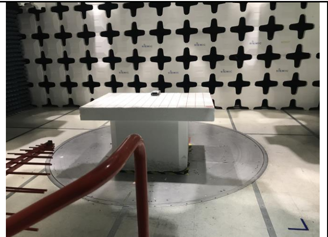
Radiated Emission Below 1G – Rear View
