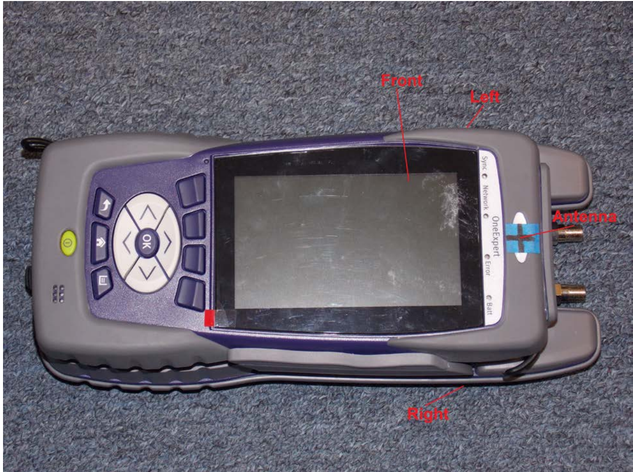
Antenna Location and Test Sides Labelled
