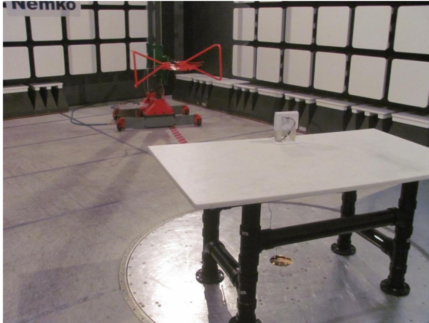
Photo 8.1-1: Radiated disturbance setup
