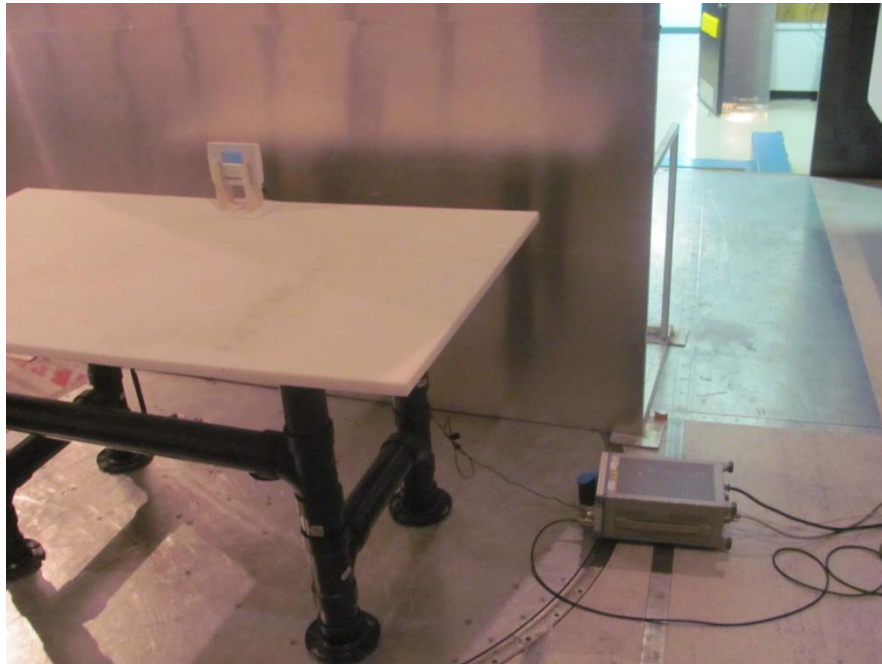
Photo 8.2-1: Conducted disturbance setup
