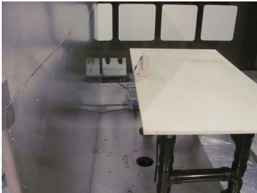
Photo 8.2-2: Conducted disturbance setup
