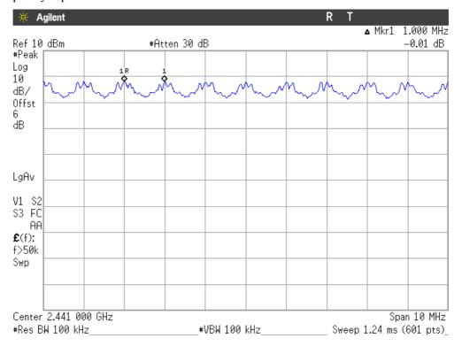
The hopping channel carrier frequencies are separated by a minimum of the two-thirds of the 20 dB bandwidth of the hopping channel
