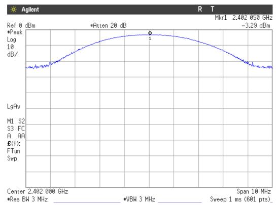
Modulation: GFSK Middle Channel: 2441 MHz.
