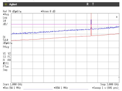
Note: The peak shown in the plot is the carrier frequency.
