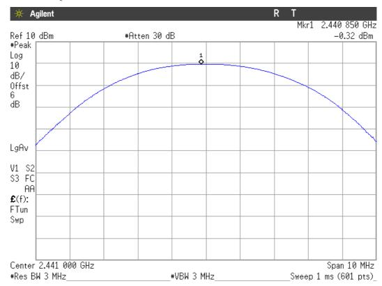
Modulation: Π/4-DQPSK Highest Channel: 2480 MHz.
