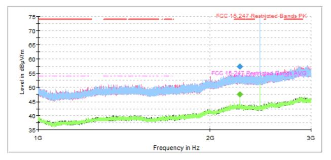
The peaks above the highest limit are the Bluetooth EDR, WLAN 5 GHz carrier frequencies.
