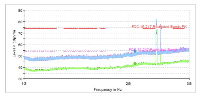
The peaks above the highest limit are the Bluetooth EDR, WLAN 2.4 GHz carrier frequencies.
