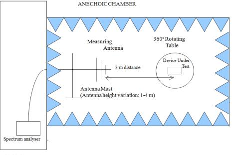
Shielded Control Room For Radiated Measurements
