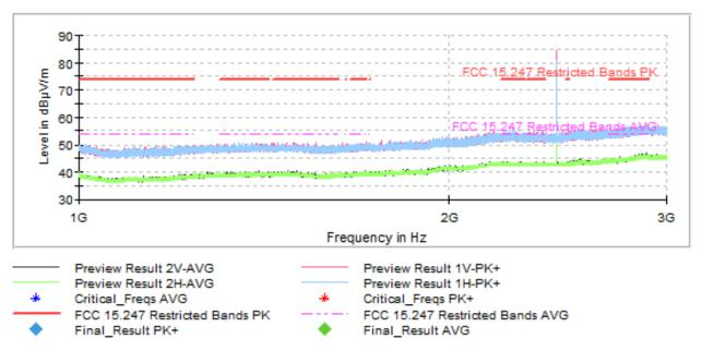
The peak above the highest limit is the Bluetooth EDR carrier frequency.
