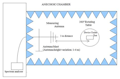
Shielded Control Room For Radiated Measurements
