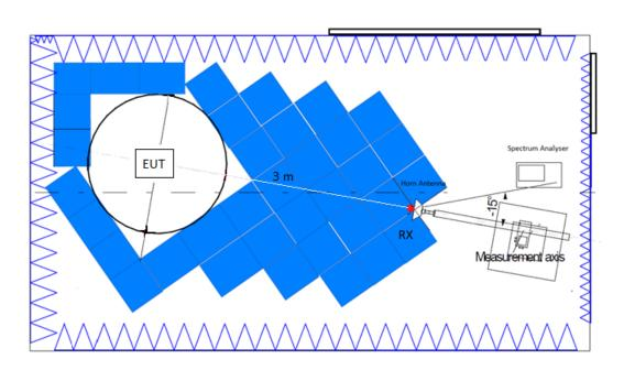
Radiated measurements setup f > 17 GHz up to 40 GHz:
