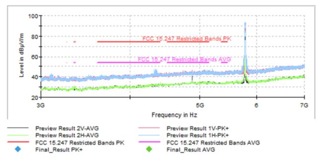
The peak above the highest limit is the WLAN 5 GHz carrier frequency.
