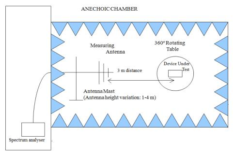
Shielded Control Room For Radiated Measurements
