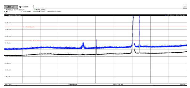
Note: The peaks shown in the plot above the limit are the carrier frequencies.
