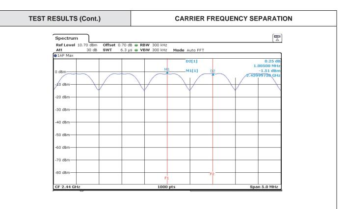
The hopping channel carrier frequencies are separated by a minimum of the two-thirds of the 20 dB bandwidth of the hopping channel.
