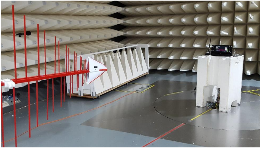
Figure B6. Radiated Emission test setup LR (0.03 – 1GHz)
