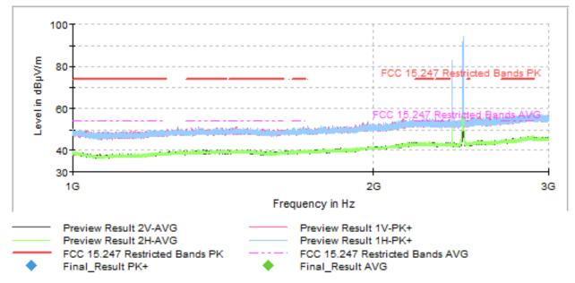
The peaks above the highest limit are the Bluetooth EDR, WLAN 2.4 GHz carrier frequencies.
