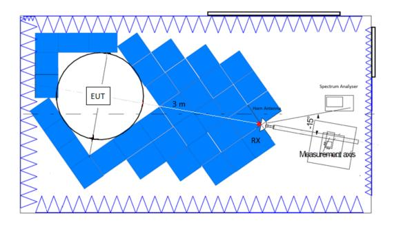
Radiated measurements setup f > 17 GHz up to 40 GHz:
