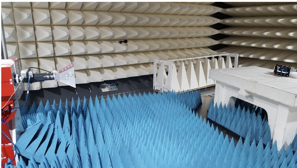
Figure B7. Radiated Emission test setup HR1 (1 – 18GHz)
