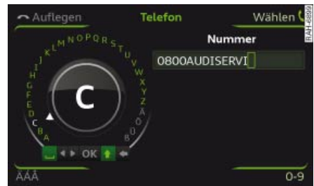
Fig. 23 Entering a telephone number via the speller for letters
