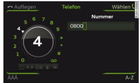
Fig. 22 Entering a telephone number via the speller for numbers
