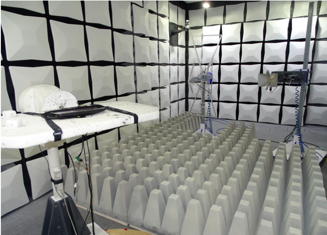
Photo 3: Test setup for radiated measurements above 1 GHz
