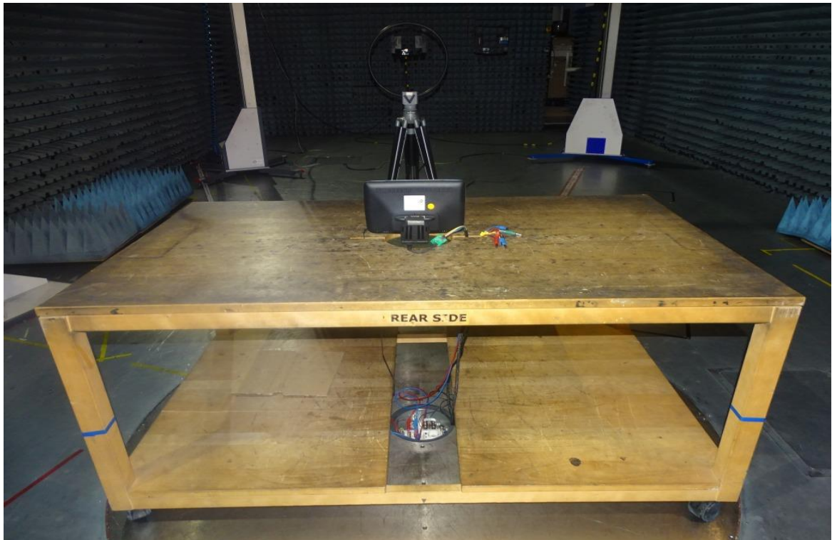
Photo 1: Test setup for radiated measurements below 30 MHz
