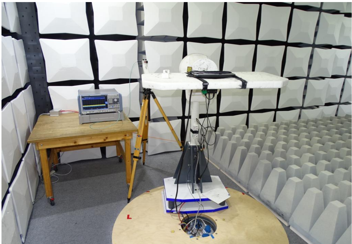
Photo 4: Test setup for radiated measurements above 26 GHz
