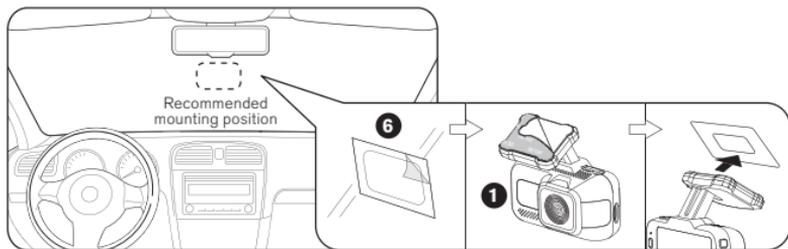
To optimize the accuracy of AI calibration, we recommend placing the Dashcam at the center of your windshield, right behind your rear view mirror.
