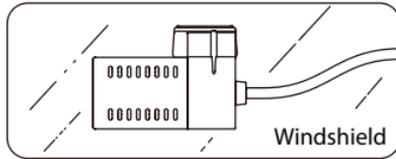
**CAUTION:** Please position the cable to the right while installing the Rear Camera to ensure proper orientation of captured images.
