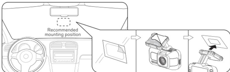
**NOTE:** To optimize the accuracy of AI calibration, we recommend placing the Dashcam at the center of your windshield, right behind your rear view mirror.
