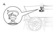
Attach the Roadcam onto the windshield. You can turn on the Roadcam and check the live screen to determine the most suitable mounting position. Utilize the knobs on the mount to tighten the suction cup.
