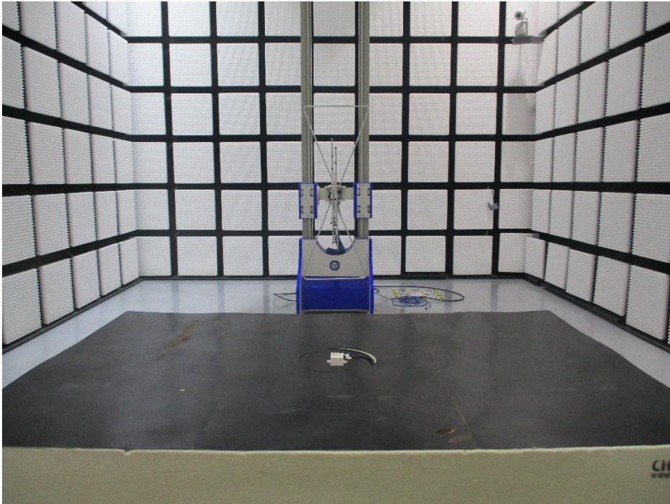
Radiated Emission test below 1GHz
