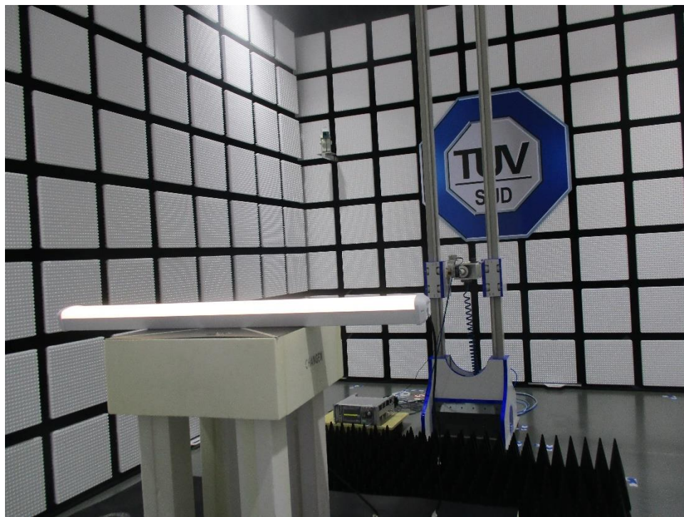
Radiated Emission test (2# Test Site) 18-40GHz
