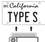
4. Peel off the cover of the double-sided tape from the International Mounting Plate, and attach the license plate to the Wireless Backup Camera
