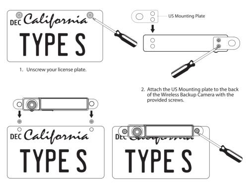
3. Using your vehicle's license plate screws, or the screws provided, align the Wireless Backup Camera with the license plate holes and secure to the vehicle.
