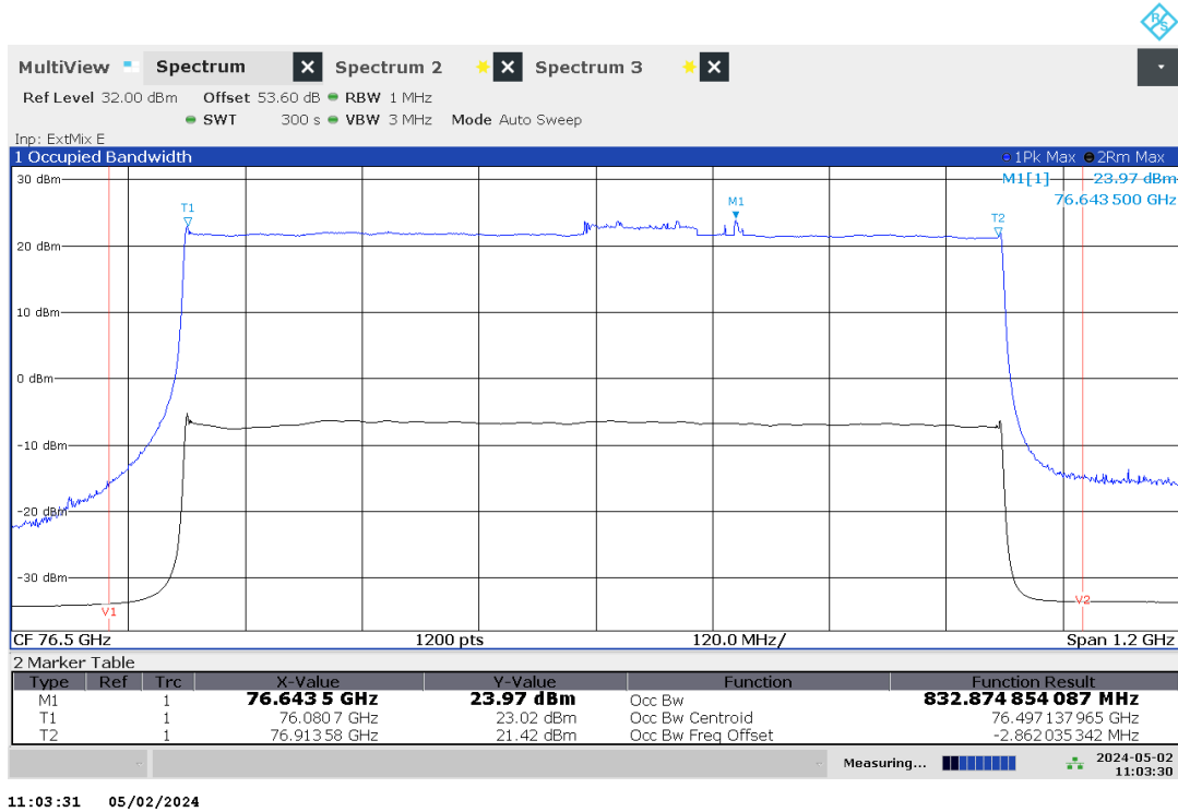
Plot no. 2: Peak Power EIRP, Peak detector
